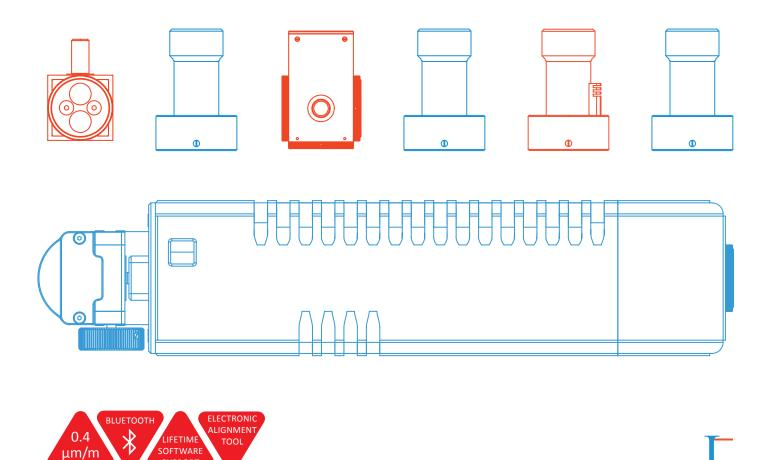
Laser Measurement System HPI-3D is the most advanced laser interferometer available on the market. Being 1 Hz two frequency heterodyne system, it offers plenty new options for users with unprecedented measurement precision and resolution. Really **easy to use**, it can be applied both in research laboratories as well as for machine geometry measurements.
